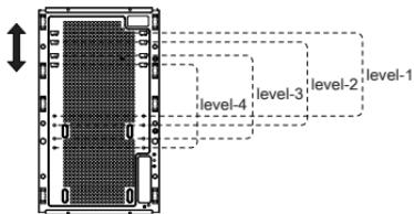
Power supply rack with 4-level height adjustment/
