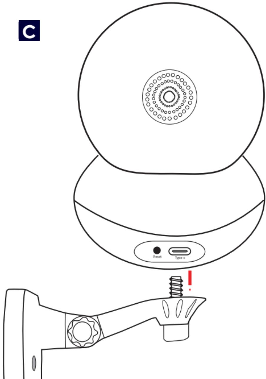
Place the camera on the screw of the mounting arm and tighten it securely
