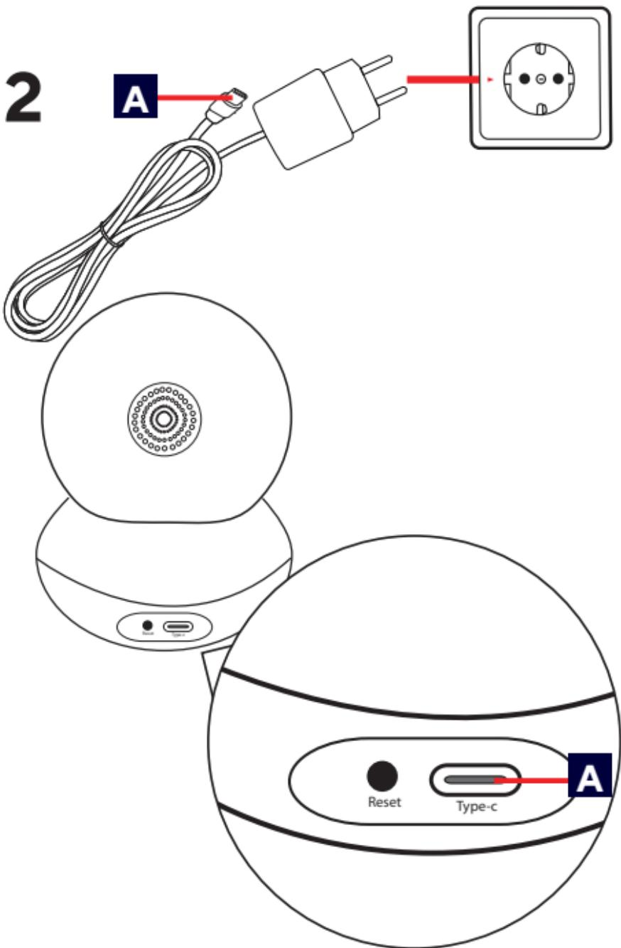
**A** Connect the supplied USB-C power cable to the back of the camera
