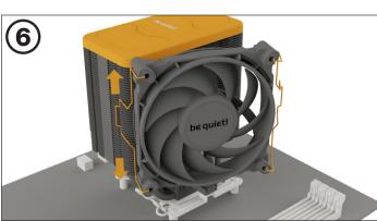
Now place the magnetic top cover on the heat sink until you hear it click into place. Use the fan clips to mount the Silent Wings 4 120mm PWM fan. You can remove the fan clips to adjust the height of the fan.
