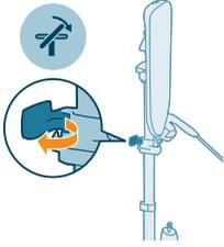
1 Unlock the board tilting lever.
