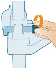
**10** Unscrew and remove the hinge knob.
