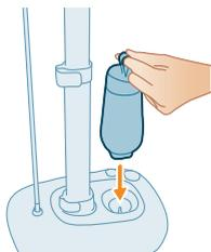
5 Insert the water tank onto the base.
