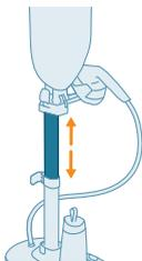
2 Push the pole down or pull the pole up to the desired height.
