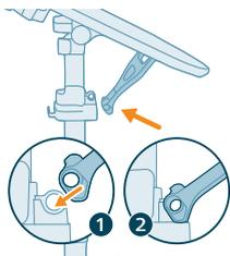
**12** Rest the Y bracket of the board onto the pole connector. The passthrough hole should be unobstructed.
