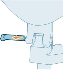
5 Remove the rod of hinge shaft.
