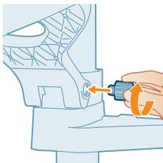
**14** Screw to tighten the hinge knob.
