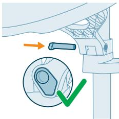
**13** Align the shape of the hinge shaft rod with the Y bracket's insert shape. Insert the hinge shaft rod through the passthrough hole.
