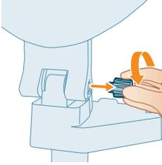
4 Unscrew and remove the hinge knob.
