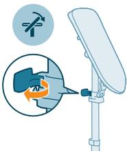
4 Unlock the board tilting lever.
