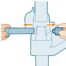
**11** Remove the rod and the hinge knob.
