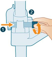
7 Insert and tighten the rod and hinge knob of the hinge shaft back to the pole connector.
