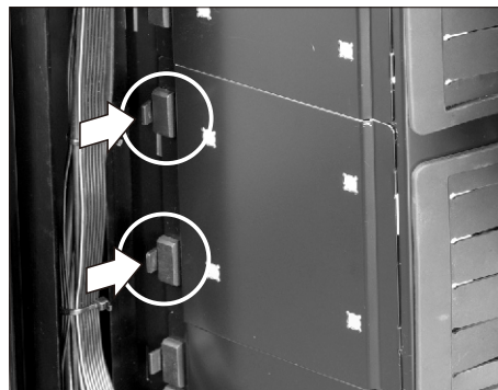
Press to release the HDD tray
