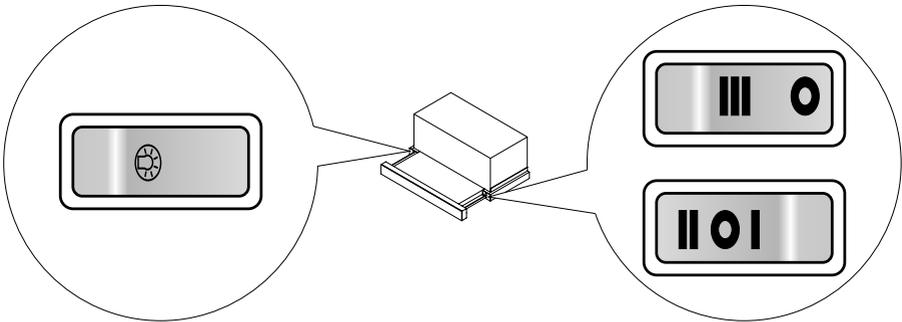
The control panel is equipped with buttons (rocker switch). You can use the buttons once the retractable front panel is ejected. Telescopic kitchen hood is equipped with a limit switch. Every time, when you eject the retractable front panel, the hood fan will start at the previously set speed.
