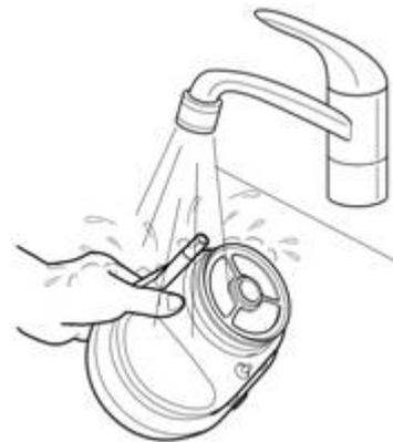
Remove the round filterinsert and clean it and the lid under running water, dry both after this. Replace the filterinsert.
