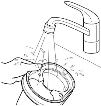
Rinse grinding/brewing container under running water and dry it after this. Clean the lid of grinding/brewing container in the same way.
