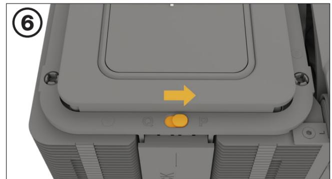
Dark Rock Elite has a Quiet (Q) and a Performance (P) mode. The mode affects the maximum fan speeds and the operating noise. To change modes, first remove the magnetic top frame. Move the switch to switch between the modes.
