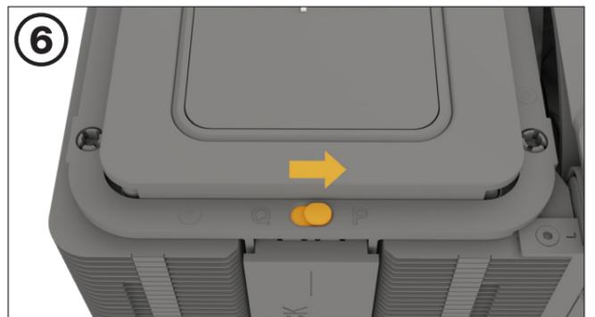
Dark Rock Elite has a Quiet (Q) and a Performance (P) mode. The mode affects the maximum fan speeds and the operating noise. To change modes, first remove the top magnetic top frame. Move the switch to switch between the modes.
