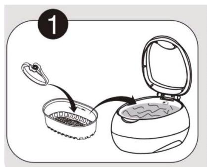
When a small item has to be cleaned, put the item into the plastic basket, then put the basket into the tank. In this way, frictions between the item and the tank can be reduced.
