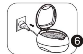
When the cleaning is finished, unplug the unit and open the lid. Take out the item. At last, pour the water from the stainless steel tank and wipe it out.
