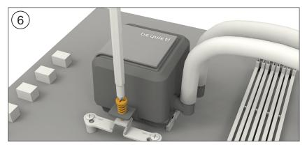
Place the CPU block centrally over the short AMD mounting brackets (5), such that these allow the CPU block to be screwed down. For this you can use a normal crosshead screwdriver. Next connect the pump to the motherboard.
