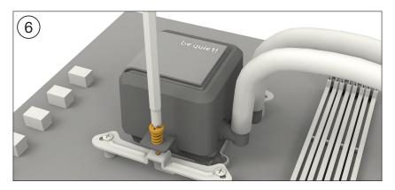
Place the CPU block centrally over the short Intel mounting brackets (4), such that these allow the CPU block to be screwed down. For this you can use a normal crosshead screwdriver. Next connect the pump to the motherboard.
