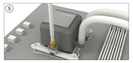
Place the CPU block centrally over the Intel mounting brackets (4), such that these allow the CPU block to be screwed down. For this you can use a normal crosshead screwdriver. Next connect the pump to the motherboard.
