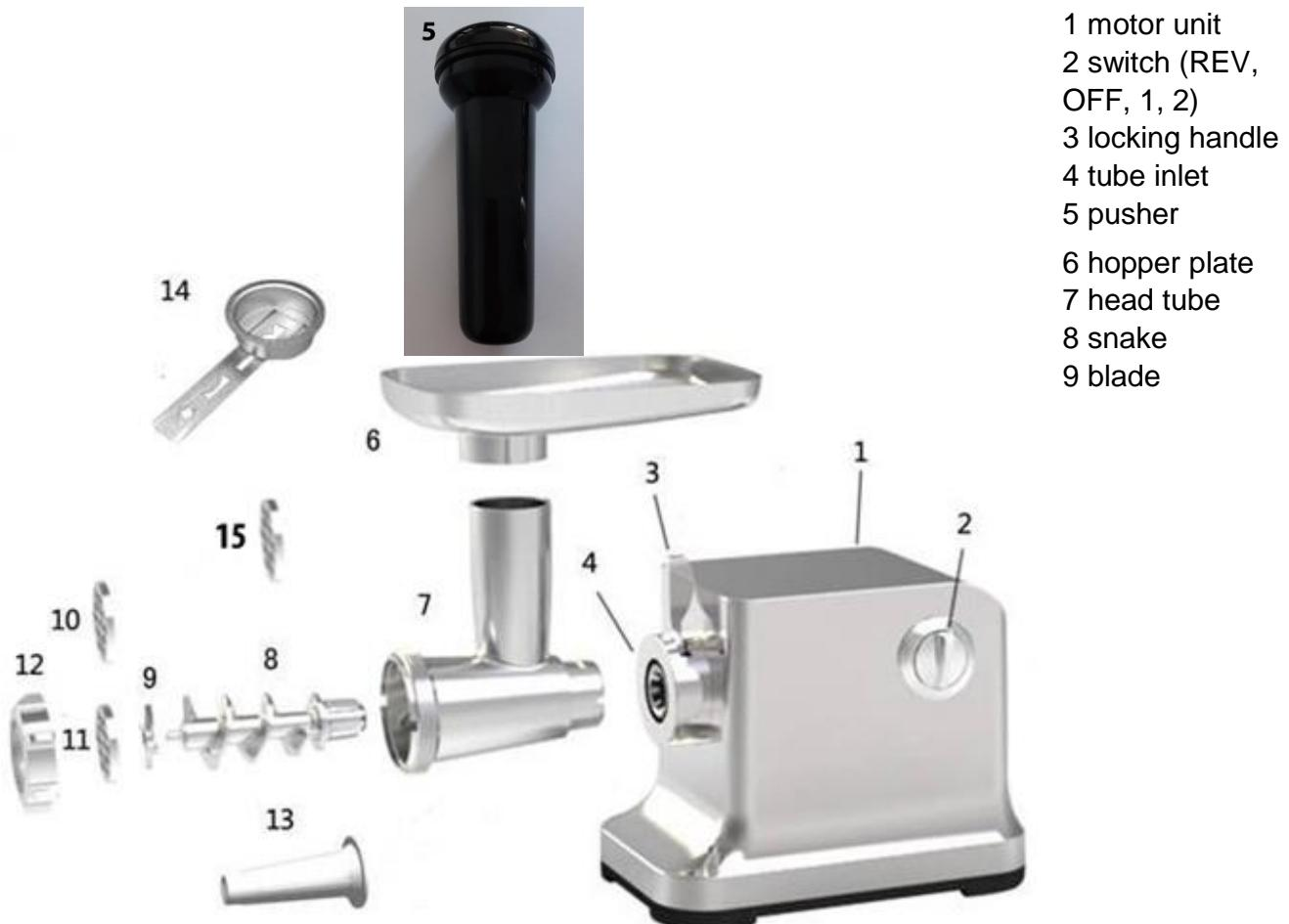
10 cutting plate medium (5mm)    11 cutting plate coarse (8 mm)    15 cutting plate fine (3 mm)
